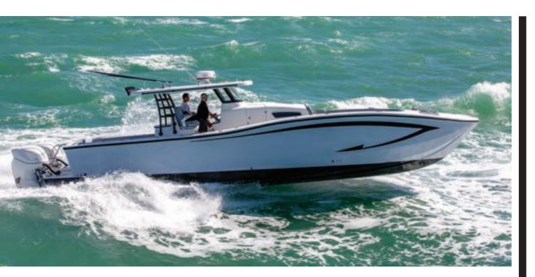
Insetta Boatworks' 45-footer is a semicustom asymmetrical cat that also features steps in its hull. **Asymmetrical sponsons** help a catamaran boat turn better, without banking outboard. Steps break surface tension. creating better speed and fuel efficiency.
