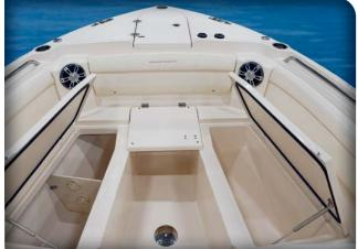
**CHECK OUT** the 32-gallon aft insulated livewell and two fish/ice boxes: one 118-qt. in the starboard bow and another 185-qt. aft.
